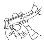
Start by holding the Poco with one hand, keeping your fingers clear of the blade's path. Place the blade flat against the wood and slowly insert it. 2.
