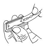
Start by holding the Poco with one hand, keeping your fingers clear of the blade's path. Place the blade flat against the wood and slowly insert it.
